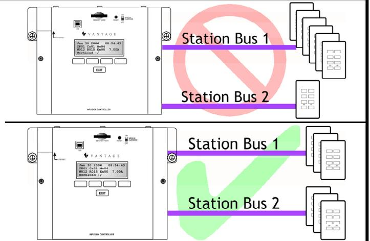
8. Daisy chain runs are fine on smaller systems, but use multiple station bus runs and tie the runs together as close to the controller as possible for larger systems. For example, in a three story house run three, separate station bus runs (one for each floor) and have them tied together as *near* the controller as possible for maximum voltage and communication at each station connected to the controller.
