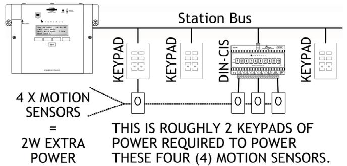
12. The Contact Input Stations, CIS and CIS10-DIN station's 12V output is rated at 50mA. This requires approximately 1.5W of power from the station bus if fully loaded. This must be taken into account manually.
