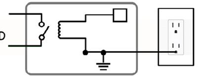
11. In Design Center individual station power specification does not account for equipment connected to the auxiliary connector. The auxiliary connector provides **12V** and is rated for **15mA**. This requires approximately **0.5W** of power from the station bus if fully loaded. This must be taken into account manually. A good practice would be to *know* the sensors power draw against the 15mA available and to not exceed that.
