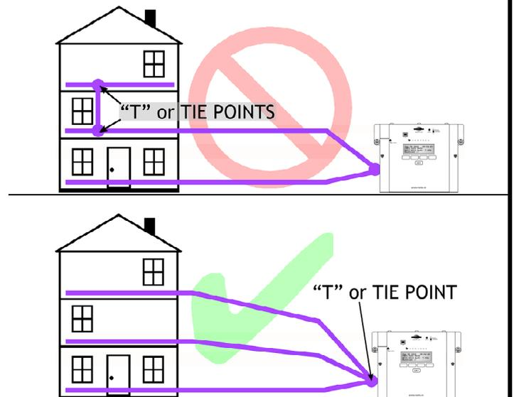
**Exception to this rule:** If the system is small enough or the "T" run is short and only adding one or two stations, the "NO" wiring example at right is an acceptable practice.
