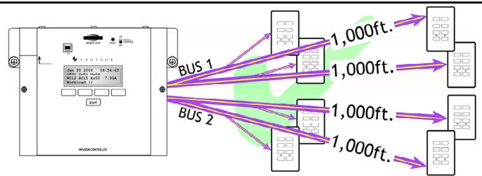
7. Design projects to balance stations on both station bus runs. For example if a single controller is configured with maximum stations and/or load power, split the stations between each bus. Real installations may not split evenly, but balancing the stations on all station bus runs helps insure better power and communication to all stations. Make sure Design Center matches the actual station bus runs if typing station serial numbers into the Design Center project.
