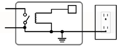
SOLUTION TO GROUNDED OUTPUT PROBLEM: ADD ISOLATED RELAY/OPTO
